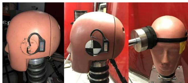
Figure 1. Mounting of the MV1, testing both an in-ear (left) and a flat mounting configuration (middle). Shown to the right is an example of a setup for right frontal impacts with a padded impactor striking from a 45 degree angle.
